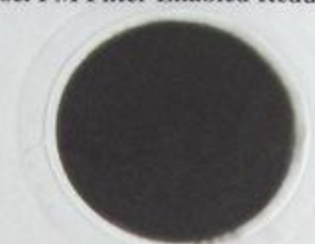
"Typical" Test Filter 0.1 g/bhp-hr
